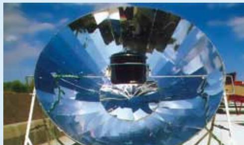
Instead of round mirrors, large solar power plants usually have parabolic mirrors in the shape of a channel or "trough." These mirrors have a focal line rather than a focal point, along which pipes carry a special liquid that is heated by the sun and that transports the heat to electricity generators.
